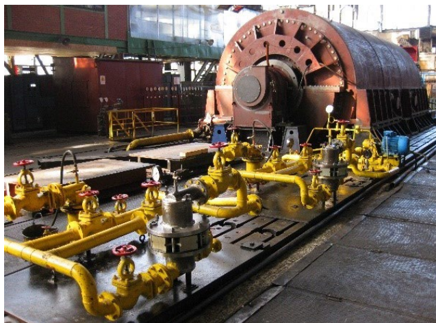
Fig. 1. Turbogenerator Type TGV-325-2AU3 on the Test Bench of the Manufacturer
