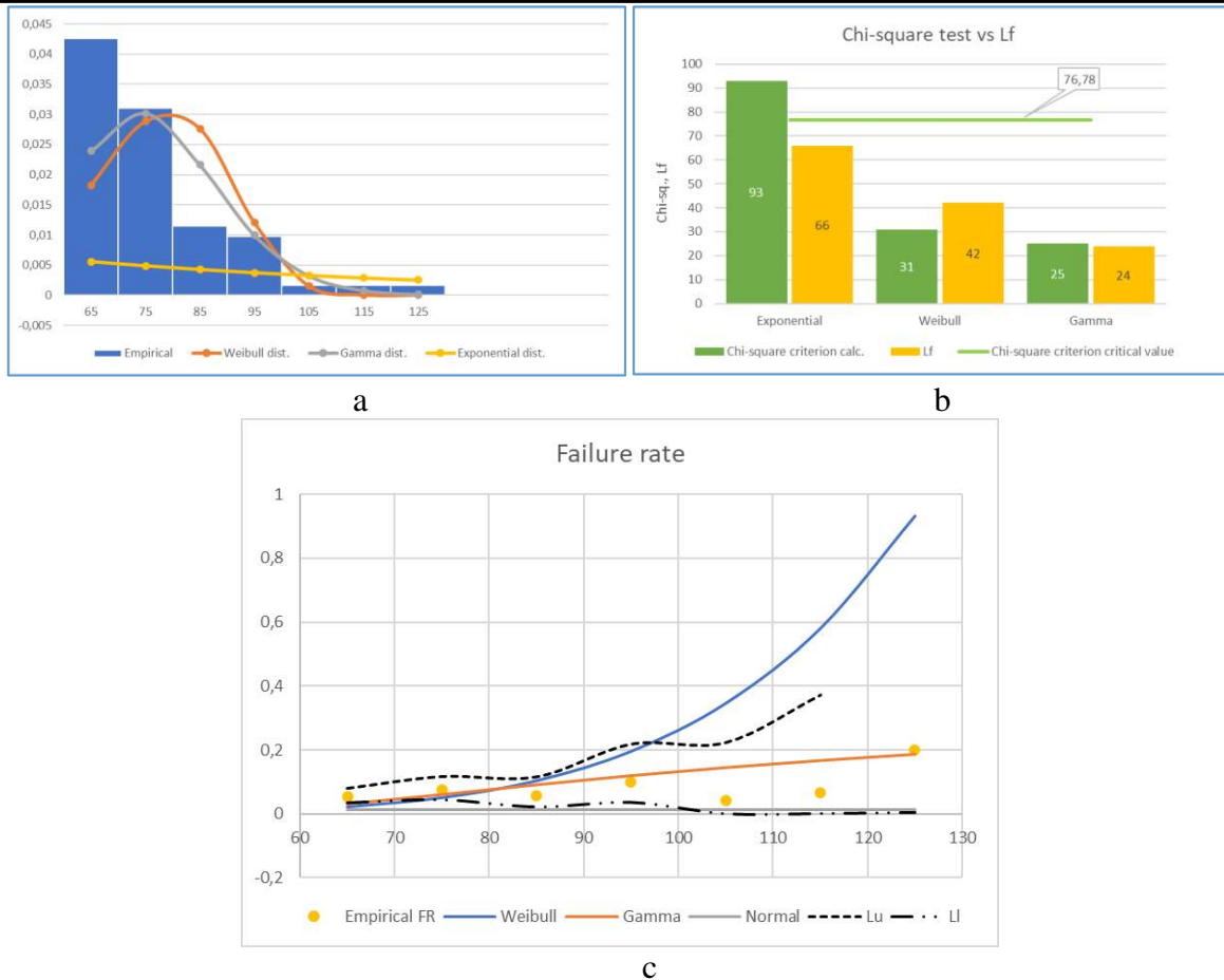
a – Empirical histogram vs theoretical distributions; b – Pearson chi-square test and L_f criterion; c – failure rates for different distribution laws Figure 4. Results of 3 mm diameter drills reliability study
